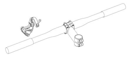
$\ensuremath{\textcircled{1}}$  Fixing DY12 on the left or right side of the handlebar and tightening the screws
