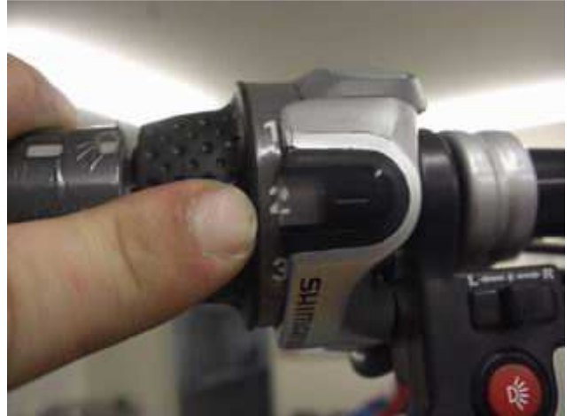
Confirm that the selector is locked in to 2 nd gear.
