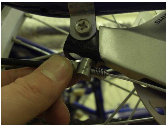
This will then lock in to place. Use this adjuster to correctly tension the rear brake
