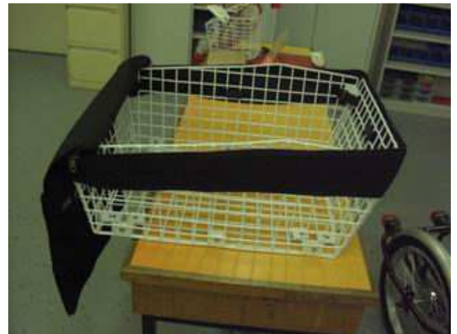
Assemble the Rear Basket. You'll find it easier if you fit the basket cover to the basket before you fit the basket to the bike
