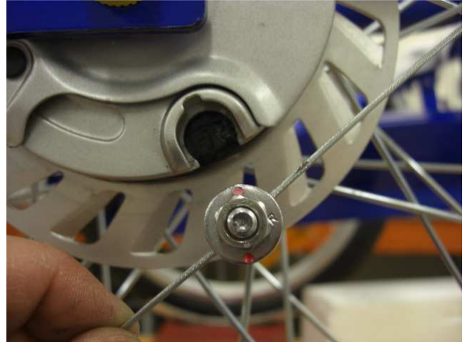
Now is a good time to connect the cables for the rear brake. These are the new Shimano Roller Brake. The brake cable is already set to the correct length.
