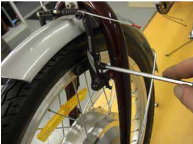
Adjust the front brakes using a 5mm Alan Key.
