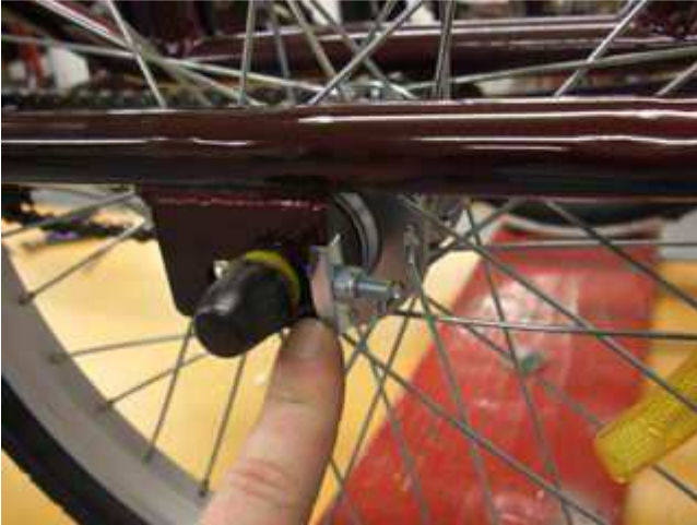
You may also need to adjust the back left hand wheel accordingly to ensure both chains are equal tension.
