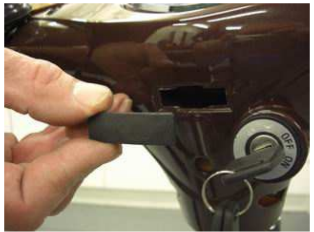
Fit supplied rubber plug to plunger bolt access hole to make appear ultra pretty . NOTE: Do not lose or damage this plug – replacement cost from Graham is $500 / from Tony is $1,000
