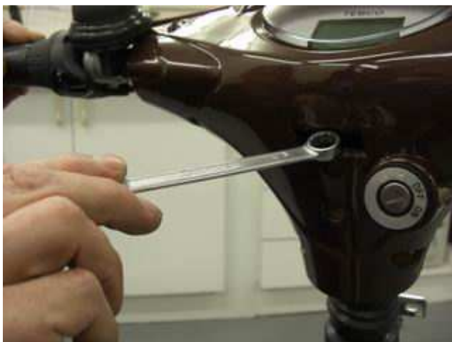
Use 13mm ring spanner to tighten head stem plunger bolt once handlebars are correctly aligned.
