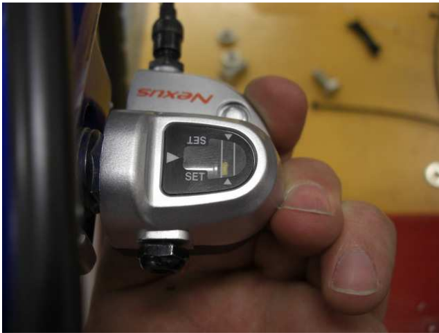
The Thick yellow line must sit between the two thin white lines when in 2 nd gear. This will correctly align the 3 gears.
