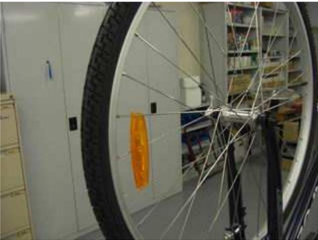
Turn the Bicycle upside down and remove the front wheel.
