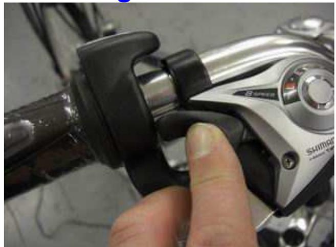
Look at the gear shifters. Ideally a trigger shift mechanism that can clear the accelerator assembly with the top selector. **Rotary gear shifters make this installation complex and messy.**
