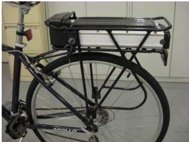
Slide the batteries in to the rack and lock in to place. Rotate the key and turn the kit on and take for a **TEST RIDE.**
