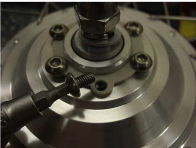
If you are using a disc brake, remove the plastic rotor spacer and use the supplied bolts **OR** make sure that the bolts used are **NO LONGER** than those supplied.
