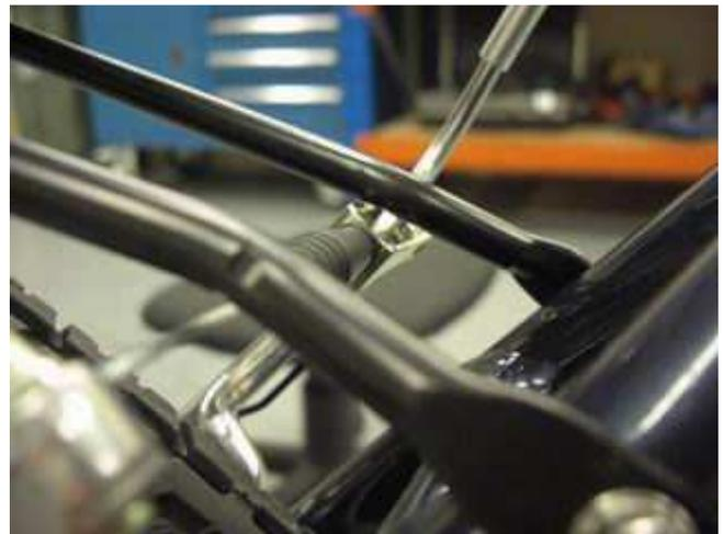
Make sure the top stays do not foul the brakes. These top rods can be bent with care to ensure clearance.
