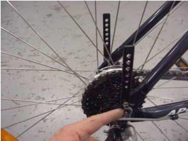
Mount the rear stays on to the frame and just nip them up. Do not tighten anything until the rack is on and levelled.
