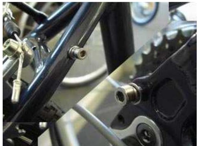
Make sure there is mounts in the frame to install the rack .
