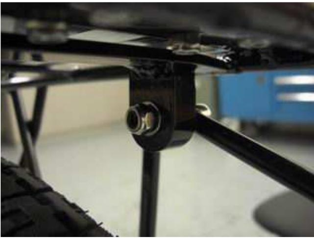
The underneath of the rack showing the top mount bolt.
