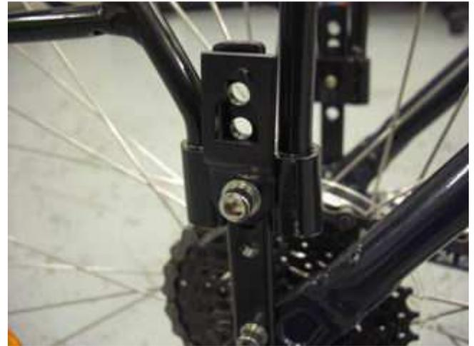
Mount the rack on the stays allowing adequate clearance over the tyre and fitting the pannier mount under the bolt.
