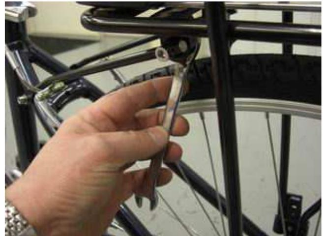
Do not wrench the head off these when tightening. If you over tighten the nut you will crack the side of the bolt where the rod passes through. Firm is fine.
