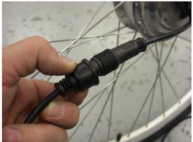
Fit the motor cable in to the plug
