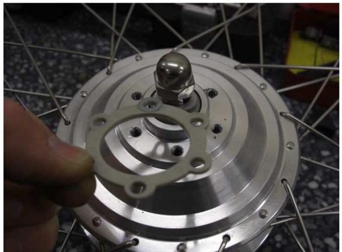
Tolerance between the housing and the internal motor is small. It is vital that the correct length bolts are used!!
