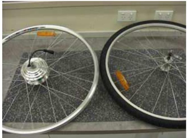
Swap the tyre from your wheel on to the motor wheel remembering that the cable comes out of the Right Hand Side
