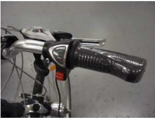
Fit the Accelerator Assembly to the right hand grip and tighten the 3mm Hex Head bolt from underneath to secure
