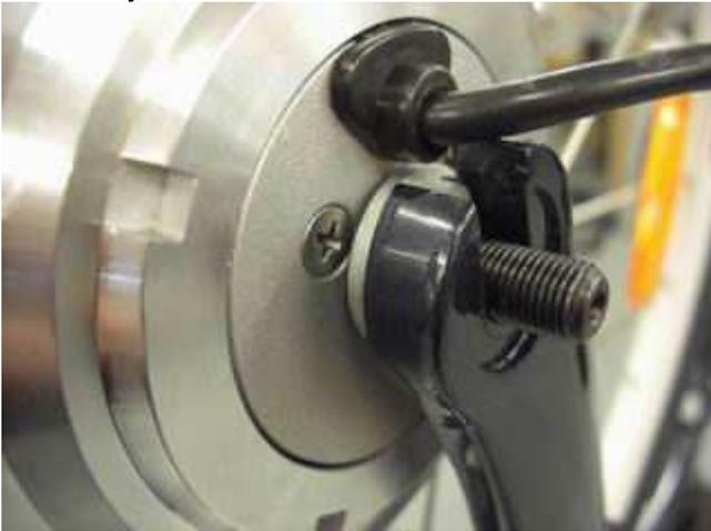
Locate the hub in to the forks making sure that the torque arm washer is in the correct place. Make sure that the motor clears the forks. If the motor is striking the forks then you will need to replace the forks.
