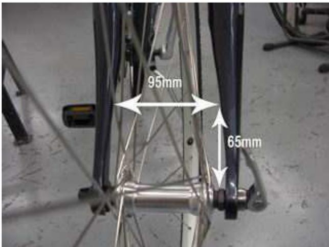
First step is to ensure that your forks are going to be compatible with the motor. You need 95mm in clearance in the width of the fork and this must extend 65mm up the fork from the axle.
