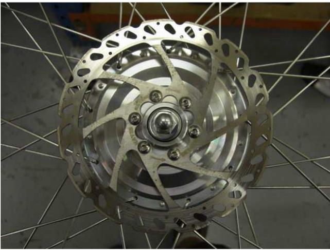
If you have disc brakes then transfer the rotor from your old wheel to the hub motor.
