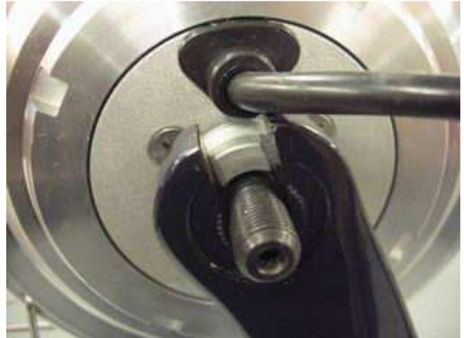
Close up of correct position – this is **CRITICAL**. The reactive rotational force of the motor is born by the fork ends. If this process is not followed correctly then the result **MAY** result in fork failure.
