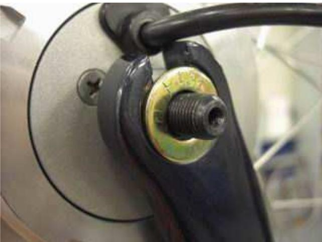
Fit the washer in to the drop out making sure that it fits perfectly.
